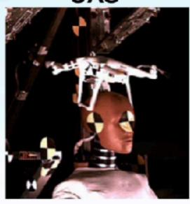
Test Weight: 2.69 lbs. Impact Velocity: 49-50 fps Impact Energy: 100-103 ft-lbs.
